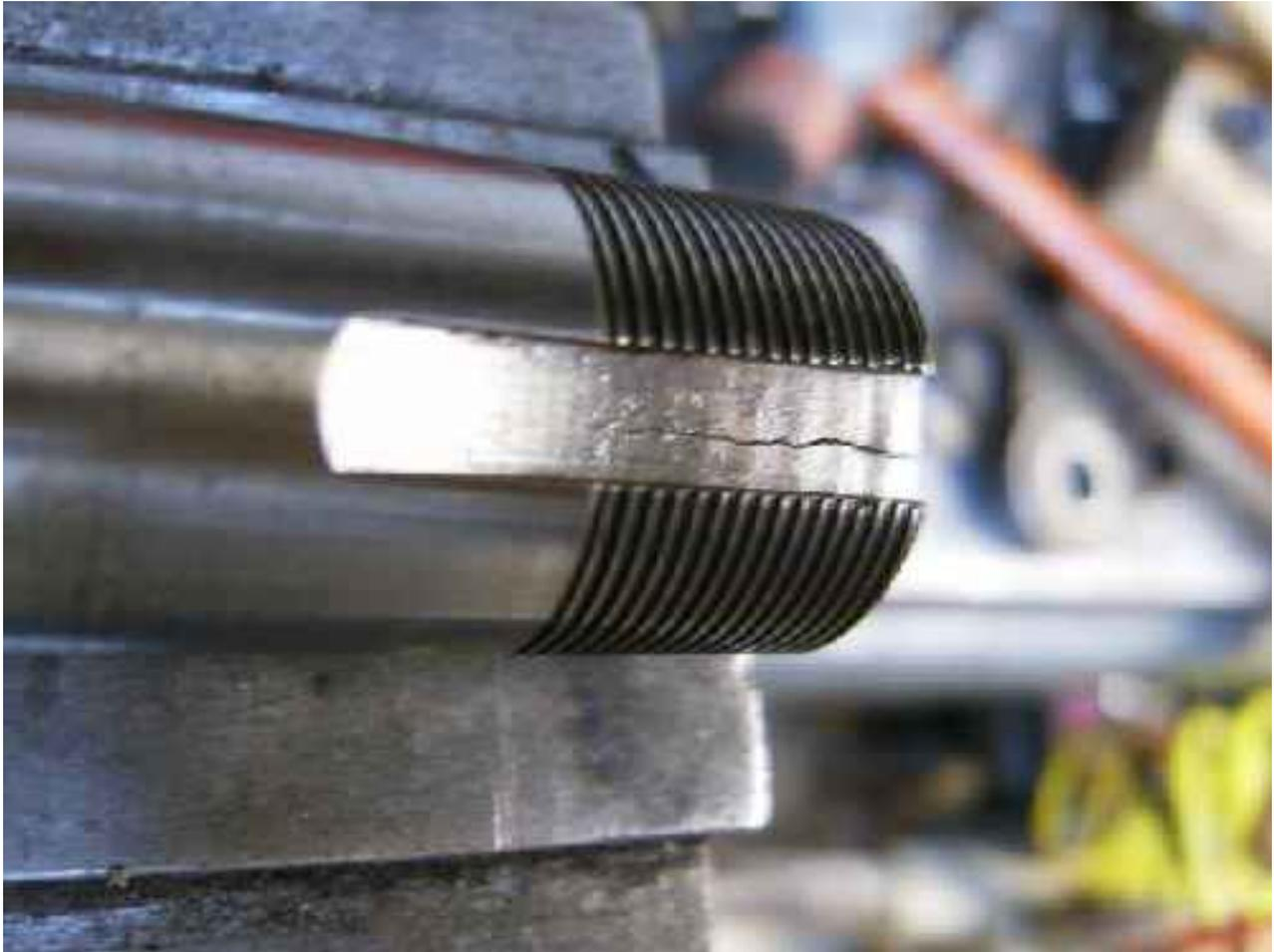
Cracked pulley end of Arbor
